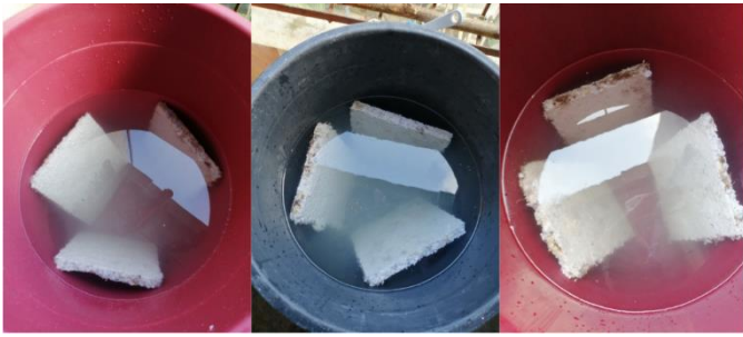
Fig. 6. GPCP composites with 10 (left), 15 (mid) and 20 (right) wt% submerged in water for 24 hours
