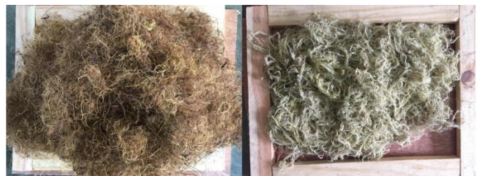
Fig. 2. Dried coir (left) and PALF (right) after the chemical retting process
